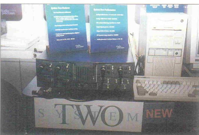
Audio Precision's new System Two. The PC-supported measurement device runs under Windows 95 and is designed to set new standards in measurement range and accuracy.
